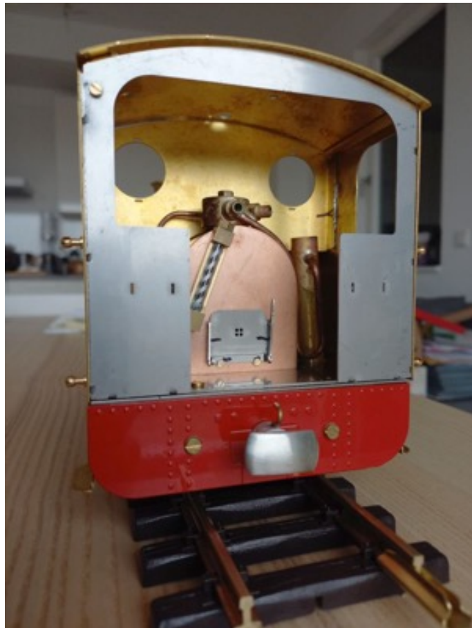
The backhead with the fire door.
