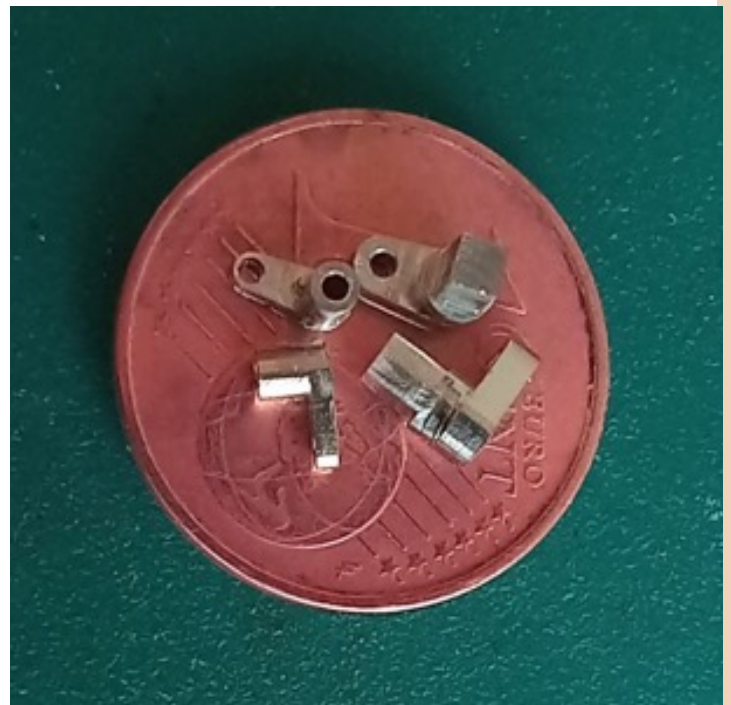
I also practiced making tiny parts with my CNC mill. These are crank pins for an H0 loco cut out of a slice of nickel silver (not yet deburred)
